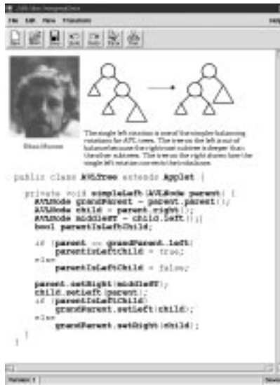
Figure 1: This screen dump of the Ensemble system illustrates how embedded multimedia documentation could be used to clarify complex algorithms, such as the rotations used to balance AVL trees. A section of Java source code is documented by a 2D graphic showing the rotation along with an explanatory paragraph. While Ensemble has in the past had support for video, this screen dump simulates an explanatory video clip with an included image.
