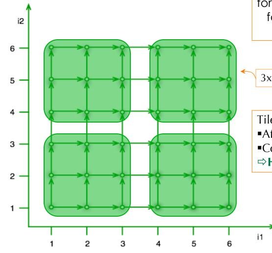
for  $i_1 = 1$  to 6 for  $i_2 = 1$  to 6  $A[i_1, i_2] = A[i_1-1, i_2] + A[i_1, i_2-1]$
