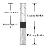
Figure 1: LRU stack is structured for the DULO replacement algorithm.
