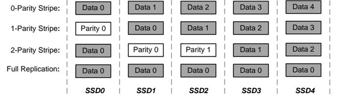
Fig. 4: An illustration of chunks and stripes in Reo.
