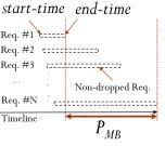
(b) Infer  $P_{MB}$  by end-time of the last non-dropped attack request subtracting end-time of the 1st non-dropped attack request during a interval.
