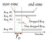
(a) Estimate  $P_D$  by start-time of the last dropped probing request subtracting start-time of the 1st dropped probing request during an attack burst.
