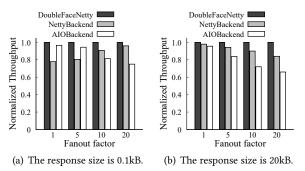
Figure 13. Normalized throughput comparison among the three servers. DoubleFaceNetty performs the best under various fanout factors and fanout query response sizes.
