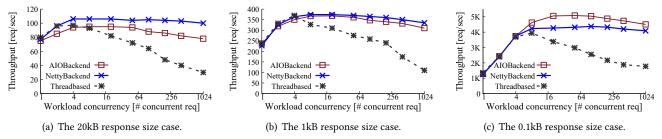
**Figure 5. Throughput comparison among different drivers for MongoDB under different workload concurrencies and fanout query response sizes.** The fanout factor is fixed to 5. Subfigures (a) and (c) show that the throughput order between AIOBackend and NettyBackend is reversed when the fanout query response size changes.
