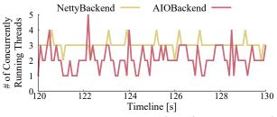
Figure 9. Concurrent running threads comparison between NettyBackend and AIOBackend.
