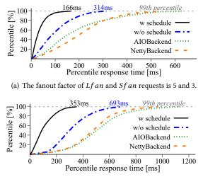
(b) The fanout factor of *Lf an* and *Sf an* requests is 7 and 1.
