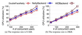
Figure 14. Overhead analysis by comparing the CPU util. at the same workload. The fanout factor keeps 20 and the fanout query response sizes are 0.1kB for (a) and 20kB for (b). DoubleFaceNetty has the lowest CPU overhead, especially at the high workload levels.
