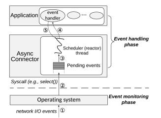
Figure 2. Illustration of a general asynchronous eventdriven connector architecture.
