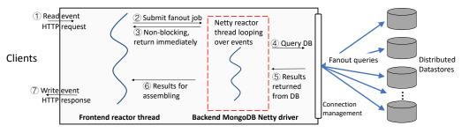
Figure 8. Architecture of the asynchronous NettyBackend server.
