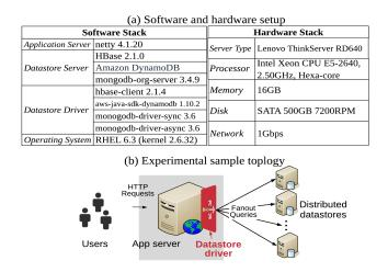
Figure 3. Details of experimental setup.
