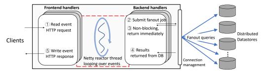
**Figure 10. Architecture of DoubleFaceNetty**. One (or a few) reactor thread is (are) responsible for managing both the events from the upstream clients (e.g., HTTP requests) and from the downstream datastores (e.g., fanout query responses).
