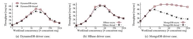
Figure 4. The performance impact of different datastore driver architectures (thread-based vs. asynchronous).
