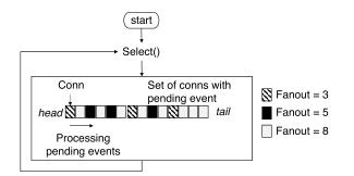
Figure 11. The completion of the client request with fanout factor 3 is delayed by events of other uncompleted requests.
