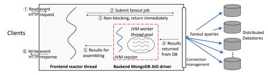
Figure 6. Architecture of the asynchronous AIOBackend server.
